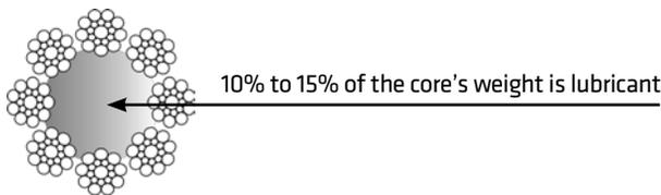
During manufacturing, a low-viscosity lubricant is applied to the sisal and strands of the ropes. The main purpose of the lubrication is to give 'life' to the rope's working parts and allow traction to take place. This lubricant also reduces metal-to-metal friction when the rope is operating and helps inhibit rust formation. It typically accounts for 10% to 15% of a sisal core's weight.
